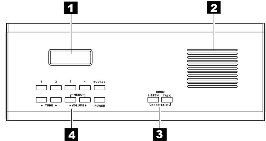
**1 DISPLAY** Easy to read Liquid Crystal Display with backlight. The display normally shows the radio frequency for AM and FM radio, but the display can also show additional important information.
