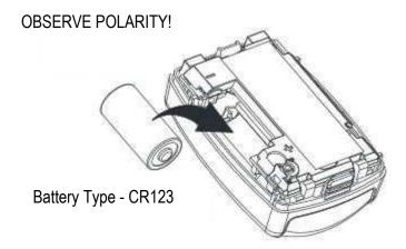
After the battery is replaced and the motion detector is back on the wall with the cover closed, you will need to enter your disarm code twice to clear the alarm event from the keypad.
